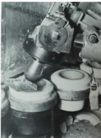
Abb.102: Jolleying in der Manufaktur Wedgwood
